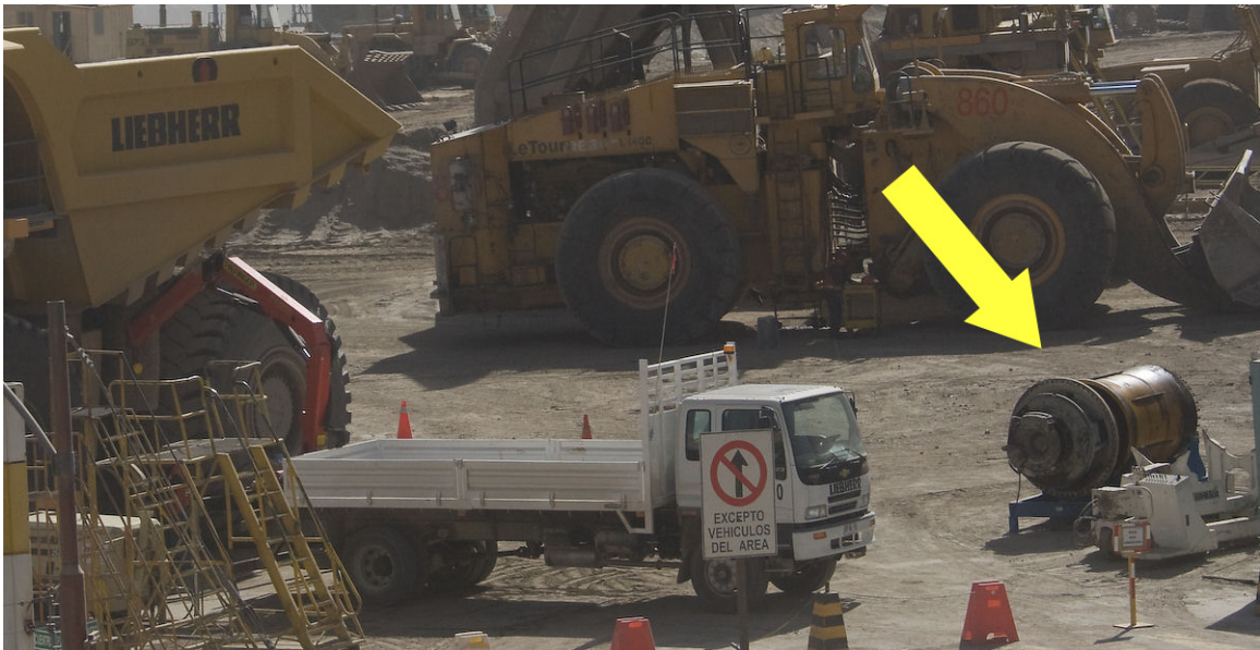
Liebherr T 282 B electric drive motor. Note boom truck for scale. Note size of brake rotor and calipers.
