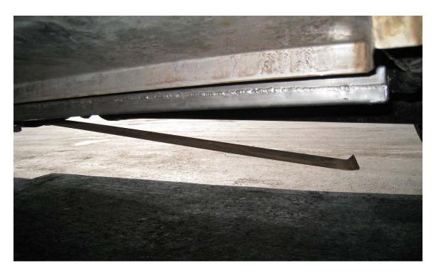
My initial view of the broken raw water tank bracket.
