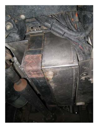
Forward end of the repaired and reinforced bracket.
