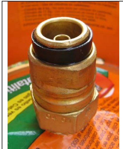
Chilean quick disconnect propane bottle connector.
