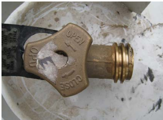
QCC Type 1 connector showing 1 5/16" / 33.3375mm ACME male threads on exterior
