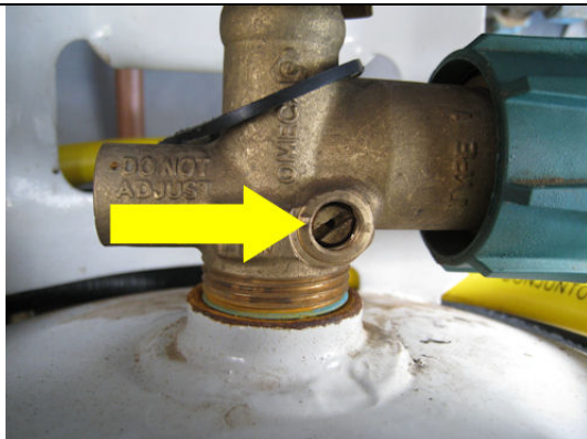
Bleeder valve on a QCC Type 1 output valve. The bleeder valve is the flat (slot) head screw.
