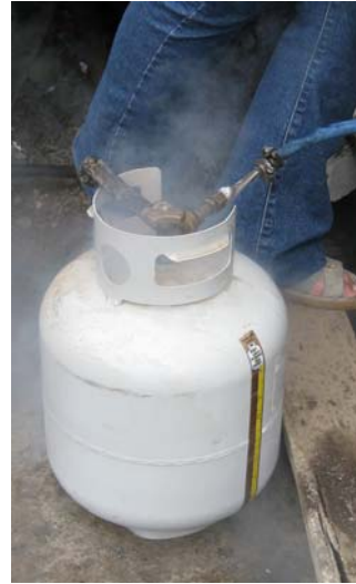
Note frost on the jumper line fitting. Liquid propane is very, very cold and will freeze your skin and tissue on contact.
