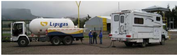
Refilling from a bobtail delivery truck. Coihaque, Chile.
