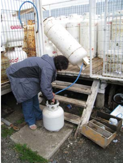
Jumper fill at Gasco bottle exchange retail location in Puerto Natales, Chile. Note inverted feeder tank.
