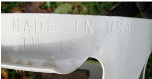
Embossed tare weight (TW) on propane bottle.
