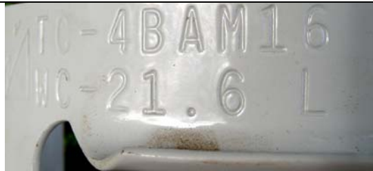
Embossed liquid/water capacity (WC) on propane bottle.
